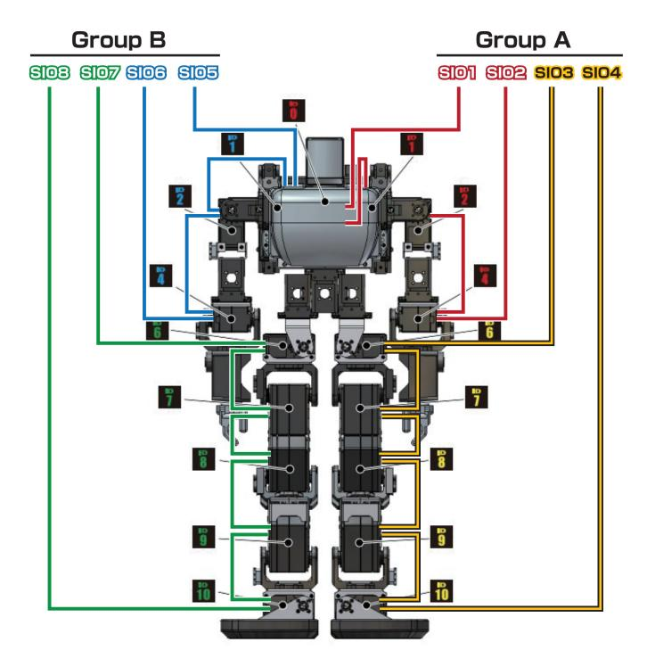
When using RCB-4mini, it is not necessary to make the servo with low maximum current consumption such as the KRS-3301 and 3302 into a loop. However, when connecting a large number of servos with high current consumption, such as the KRS-3304, it may be necessary to return the end servo to the RCB-4mini in a loop.
