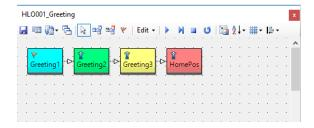
16. The number of lines that can be drawn coming out of a control is one, or two for a branch control. There are no limitations to the number of lines that can be connected into a control.
