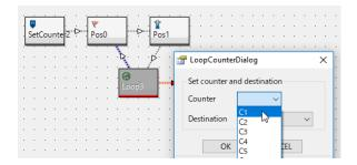
In the LoopCounter control, the set counter value is reduced by 1 and when it reaches 0, the process moves to the control specified as the destination. The LoopCounter control initially subtracts 1 and then shows the result, so to repeat 5 times, set the SetCounter control to 6.
