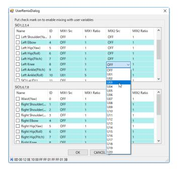
A user variable must be specified. When a value is substituted in the user variable by other motions (SetValue control), the mixing result of the specified servo changes. For example, if the U01 user variable address is set to x 3 by the URemix control and 10 is set for U01 in the SetValue control, the servo selected by the URemix control will be subjected to mixing of U01 x 3 = 30.
