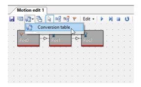
3.A Conversion Table screen will be displayed. Click on the operation field of the target servo, display the conversion menu and select a conversion function. The screenshot shows an example of producing a symmetric movement in the upper body.
