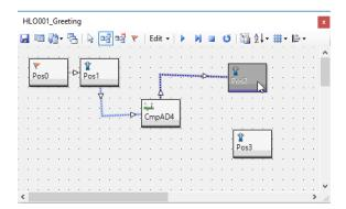
8.To connect to a destination for when branch condition is met, use the branch connection mode. By switching to the branch connection mode and connecting a line to another control, the branched line turns red. In the figure, the connection is created so that when the conditions set in CmpAD control is met, the program proceeds to Pos3, and when the condition is not met, the program proceeds to Pos2.
