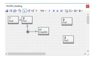
6.Switch to connection mode. In the connection mode, by drawing out a line from the branched control, a line for when condition is not met can be connected. Click on the screen while a line is being drawn to turn it into an anchor point. The line and anchor point can be canceled with the ESC key.
