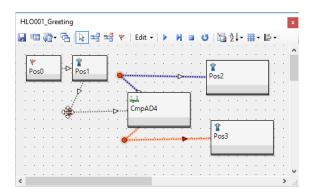
13. Dragging the Edit Screen while pressing the ALT key will scroll the screen.
