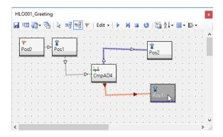
9.Switching to the selected mode with the ESC key displays round anchor points. By areaselecting, anchor points can be selected, too.
