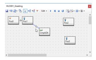
4.Clicking on the anchor point selects the anchor point. Press the DEL key while it is in a selected state to delete the anchor point.
