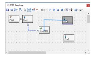
7.Click on a destination to complete connection of line for when branch condition is not met.
