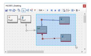
10.Multiple controls can be moved by pressing the SHIFT key.
