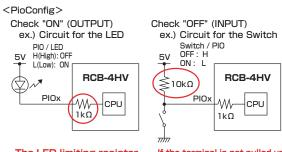
The LED limiting resistor is mounted on the RCB-4.
