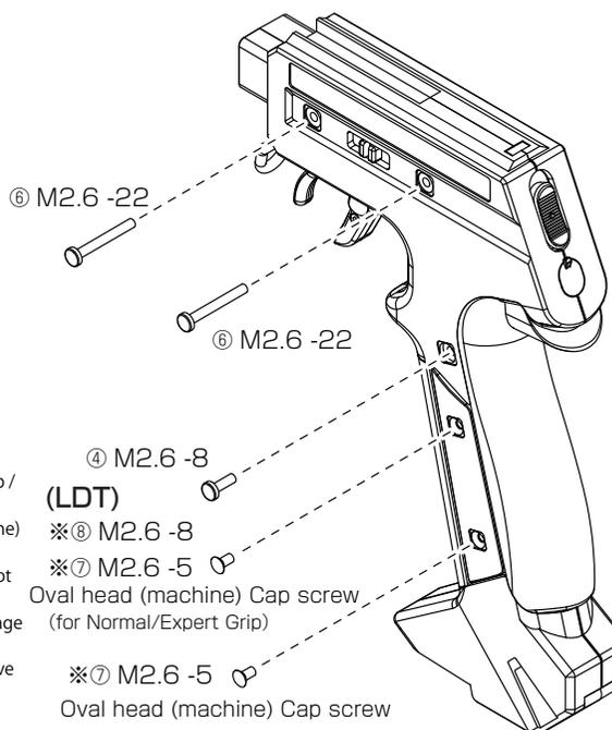
※If you use the large grip / LDT, please use the ⑧ M2.6-8 oval head (machine) Cap screw. If you use normal/expert grip, do not use this screw. Using the incorrect screw can damage the battery box and you may not be able to remove the battery case.
