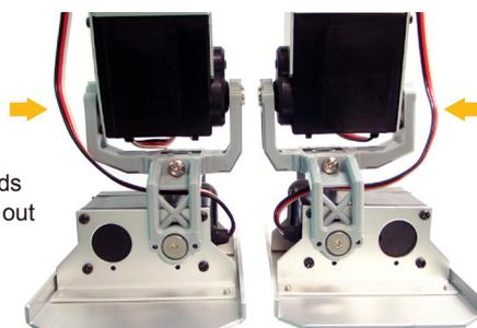
CH15, CH21 servo leads (arrows) should be put out through the under side of the servo arm.
